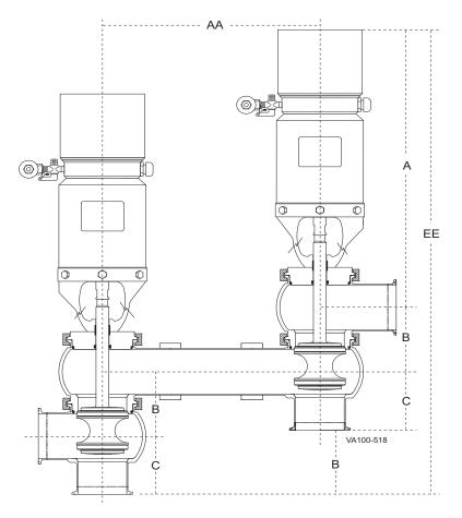
Figure 3: Valve Dimensions
