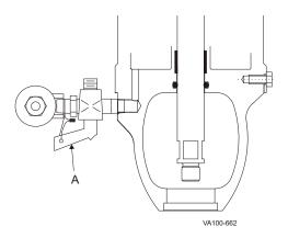
Figure 24: Air Shutoff Valve
