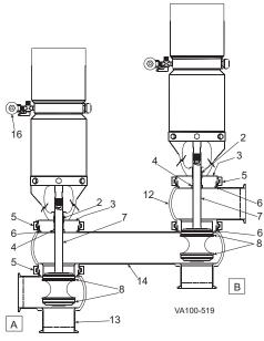
A. Divert Valve B. Leak Detect Valve
