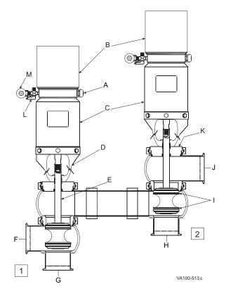
Figure 1: Flow Diversion Valve Nomenclature
