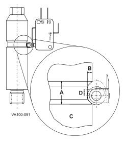
Figure 13: Detail of the Micro Switch
